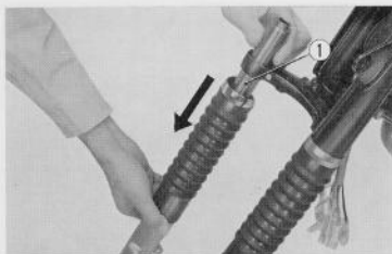
Fig. 4.29 Removing front fork assembly ① Front fork
