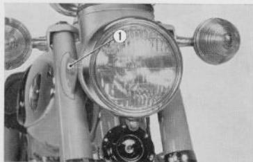
Fig. 4.25 Removing headlight ① 8×22 hex bolt
