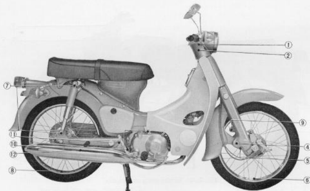
Fig. 5.44 Torquing points on right side
