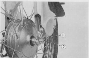
Fig. 4.33 Removing front wheel ① 8×22 hex bolts ② front wheel axle
