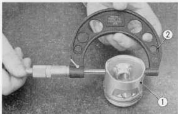
Fig. 3.52 Measuring piston skirt diameter ① Piston ② Micrometer
