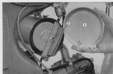
Fig. 4.67 Removing air cleaner mounting bolts (S 90) ① Air cleaner case cover ② Air cleaner mounting bolt
