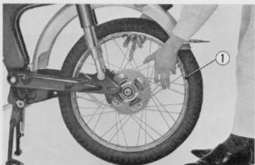
Fig. 4.73 Removing rear wheel ① Rear wheel
