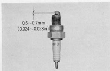
Fig. 5.10 Measuring spark gap
