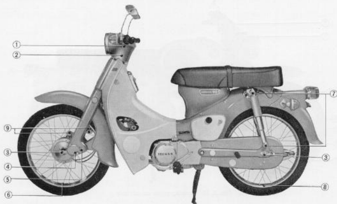
Fig. 5.43 Torquing points on left side
