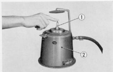
Fig. 5.9 Spark plug cleaner ① Spark plug ② Spark plug cleaner
