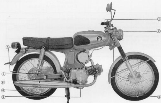
Fig. 5.40 Torquing points on right side
